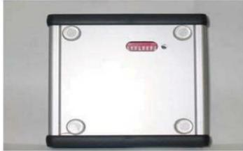
**Dip Switches:** These switches are used to control the tone, the sound of the tone and the calibration mode.
