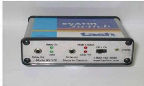
**Relay Out:** Plug the relay cable into this port. It connects directly to the device you want to control.
